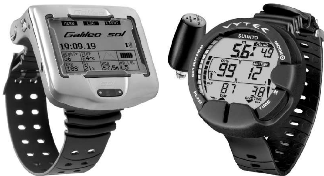
Figure 4.3 Two of the more sophisticated current model recreational dive computers (a) Galileo Sol (Scubapro, USA); and (b) Vytec (Suunto, Finland).
