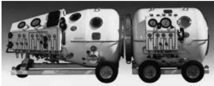
Figure 68.2 Portable, lock-on, two-person recompression chambers. A side view of the chamber system built by Cowan Manufacturing for the US Navy and the Royal Australian Navy. The cone-shape treatment chamber is shown next to the cylindrical transfer chamber. When the two chambers are joined together, they can be operated as a two-compartment chamber. (Courtesy of Cowan Manufacturing, Warners Bay, Australia.)
