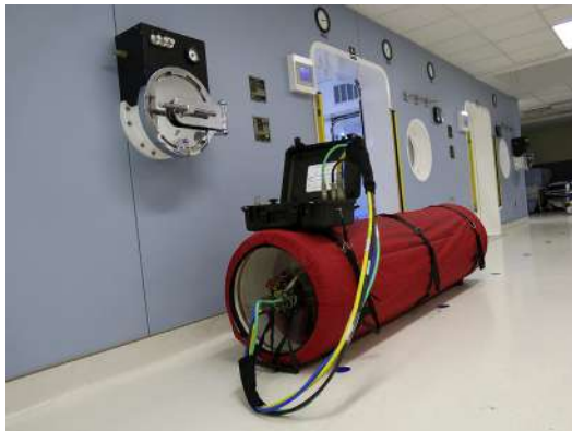
Fig. 7. A hyperbaric stretcher set up in front of a multiplace, multilock hyperbaric chamber. (Courtesy of D. Buteau, MD, Quebec City.)
