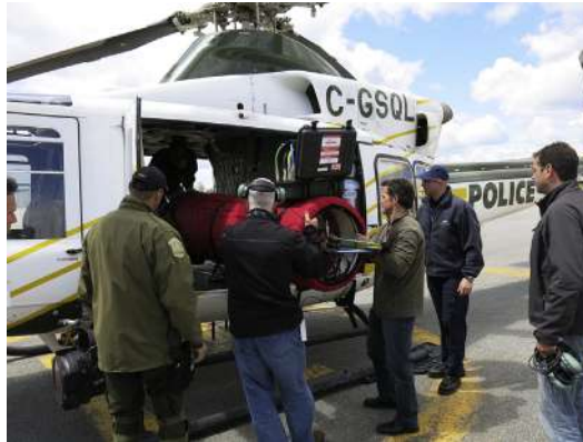
Fig. 8. A hyperbaric stretcher being loaded onto a helicopter. (Courtesy of D. Buteau, MD, Quebec City.)
